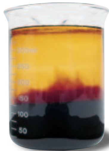
Figure 6.14 The random movement of molecules of corn syrup and water will cause the uncolored sample to diffuse into the colored sample.
